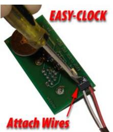
Can access the wiring (there should be 3 actuator wires - red, black and white)
